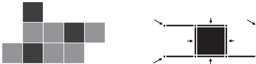
Figure 5. Some full cubes that can be removed from the cubical set are shaded dark at the left-hand side. Free faces are indicated with arrows at the right-hand side.
